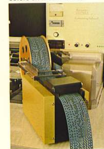
JACQUARD CARD READER: Jacquard card inventory can be utilized by reading into memory and operating at high speed. (Optional)
