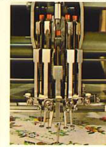
JUMP STITCH: The jump stitch is utilized for spectacle framing for those stitches more than 12.7mm.
