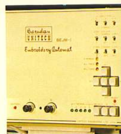
IC MEMORY: Standard capacity is 32,000 stitches. Additional memory optional to increase to a maximum of 160,000 stitches.
