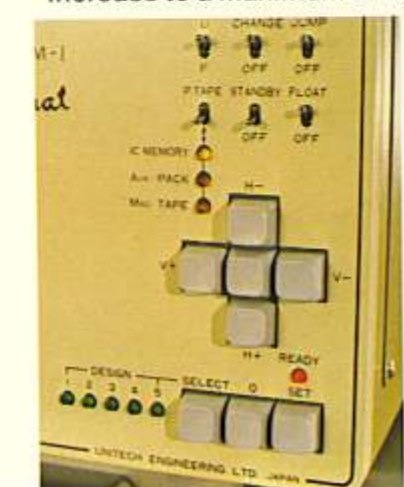
RANDOM NEEDLE SELECTION: The arrangements of colors in a pattern can be changed as desired to utilize the full five colors on the machine.
